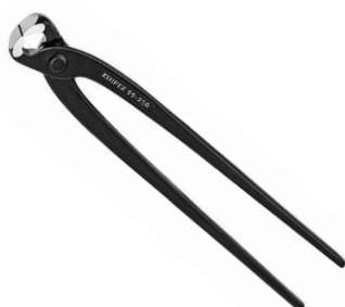
KPX9900250 Knipex Concrete Nipper 250mm • Cutting capacity medium hard wire: 2,4 Ø mm • Cutting capacity hard wire: 1,6 Ø mm
